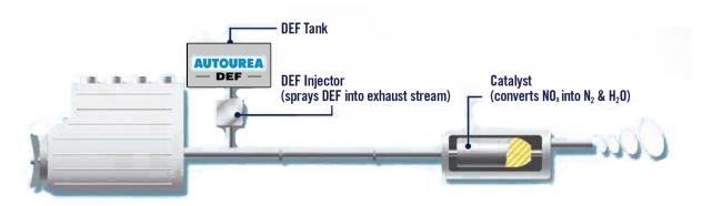
SCR technology reduces the concentration of nitrogen oxide (NOx) gases that are produced inside the engine during combustion. This process requires the right amount of DEF to be injected into the exhaust stream. Upon mixing with exhaust gases, it is hydrolyzed before the catalytic converter breaks down nitrogen oxide (NOx) into harmless nitrogen (N2) and water (H2O).
